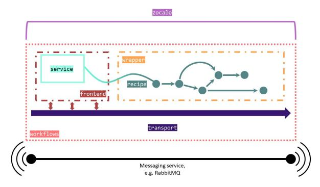
python-workflows interfaces directly with an externally provided client library for a message broker such as ActiveMQ or RabbitMQ through its transport module. Services then take messages, process them, and maybe produce some output. The outputs of services can be piped together through a recipe. Services can also be used to monitor message queues. python-zocalo runs python-workflows services and recipes, wrapping them so that they are all visible to Zocalo.
