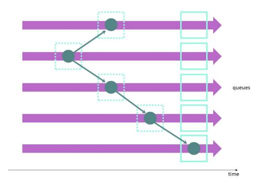
This diagram illustrates the overall task management model of Zocalo. Services run continuously, consuming from the relevant queues. Recipes inside of wrappers dictate the flow of data from queue to queue and, therefore, from service to service. The nodes represent input data which is given to the service with the output of a service becoming the input for the next.
